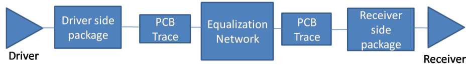
Figure 53. Equalization network to improve the insertion loss profile of the signal and minimize SSN induced jitter and noise
