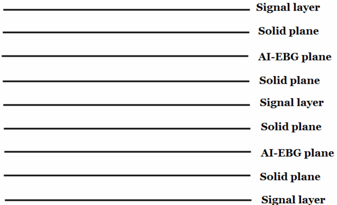
Figure 5.27 Plane stack-up for multilayer structure for avoiding possible problems related to signal integrity and EMI.
