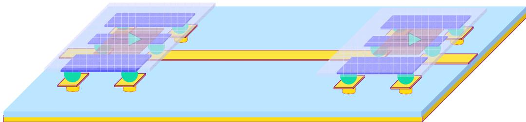
**Figure 7.2** wafer-level package test vehicle including integrated circuits.
