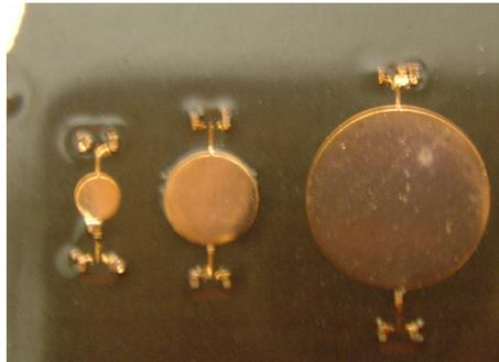
**Figure 2.23** Capacitors fabricated at PRC.
