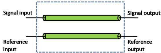
Figure 89. Four port transmission line model.
