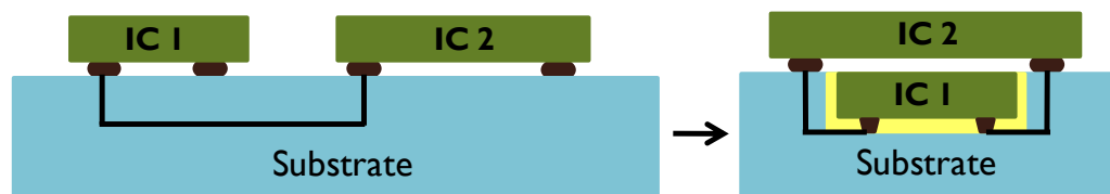
Figure 12 Increase in functionality with smaller package size as benefit of chip-last embedding
