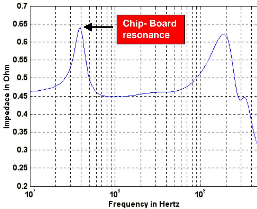
Figure 7.10(b) Self- impedance from the chip attached to board
