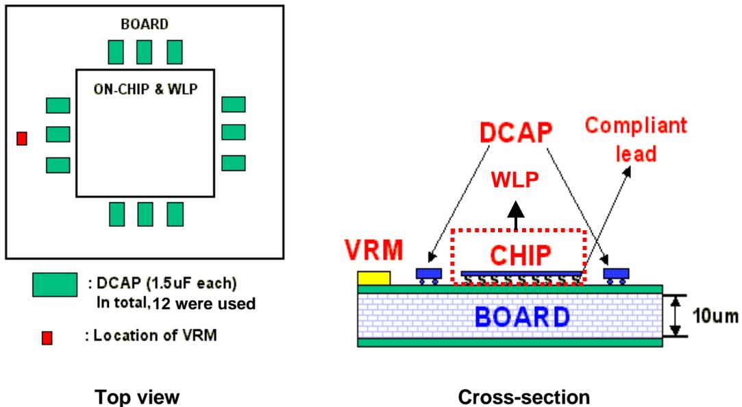
Figure 7.6 Board with 12 decoupling capacitors and a wafer level package
