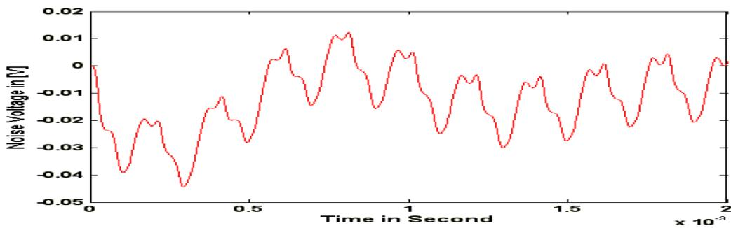
Figure 7.2(d) Differential noise at a CMOS inverter
