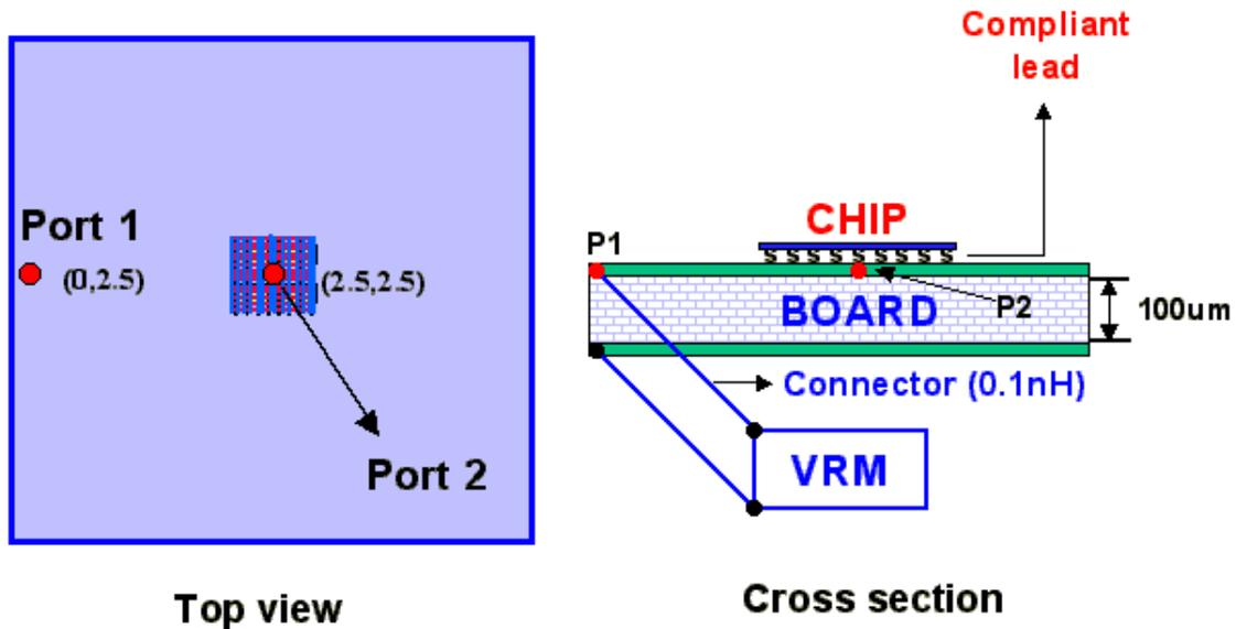
Figure 7.8 Plane pair with an on-chip power grid
