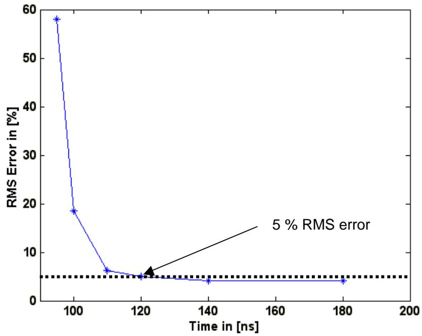
Figure 6.9(a) RMS error with the variation of the time duration
