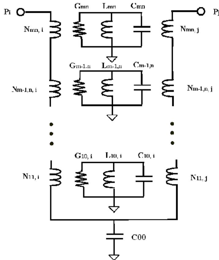
Figure 5.4 Equivalent circuit of the plane model for two arbitrary ports
