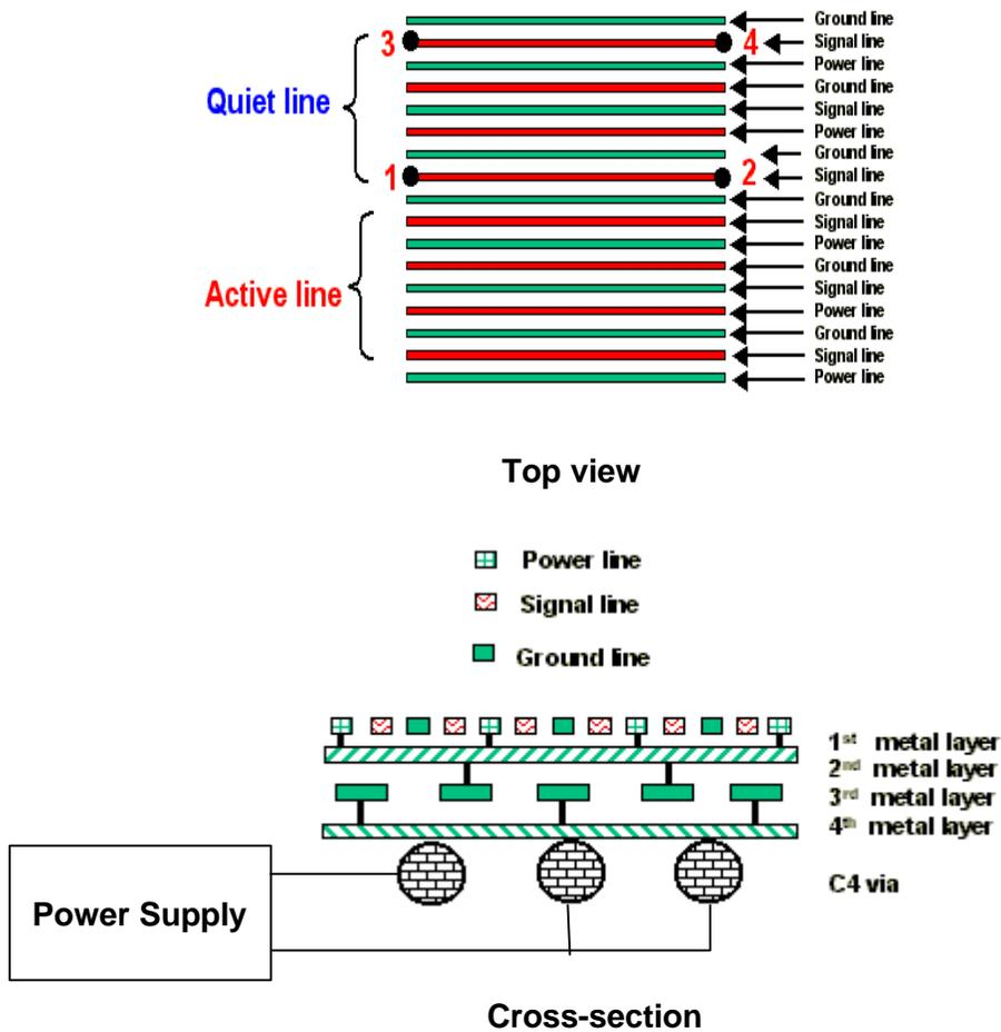
Figure 4.10 On-chip bus structure in power grid
