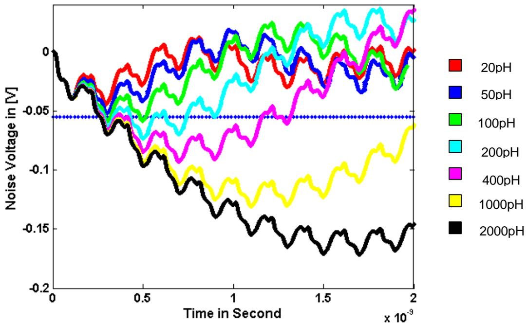
Figure 7.3 Differential noise from the power grid structure with the variation of compliant interconnect inductance from 20pH to 2nH
