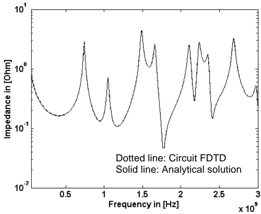
Figure 6.8 (b) Trans-impedance at Port 3 from the open structure
