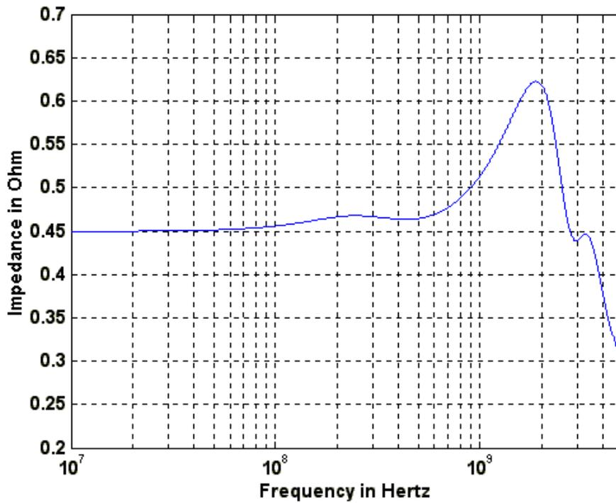
Figure 7.10(a) Self-impedance seen from the chip only
