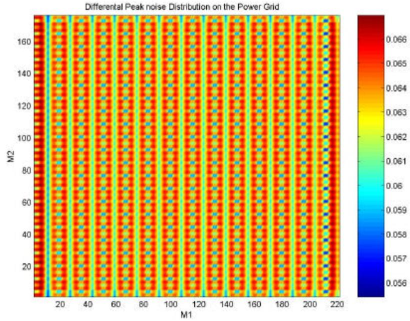
Figure 2.8 Differential peak noise distributions under uniform current distribution
