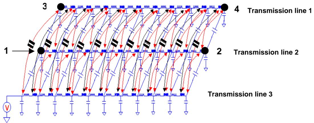
Figure 4.4 Coupled transmission lines with mutual inductance and capacitance
