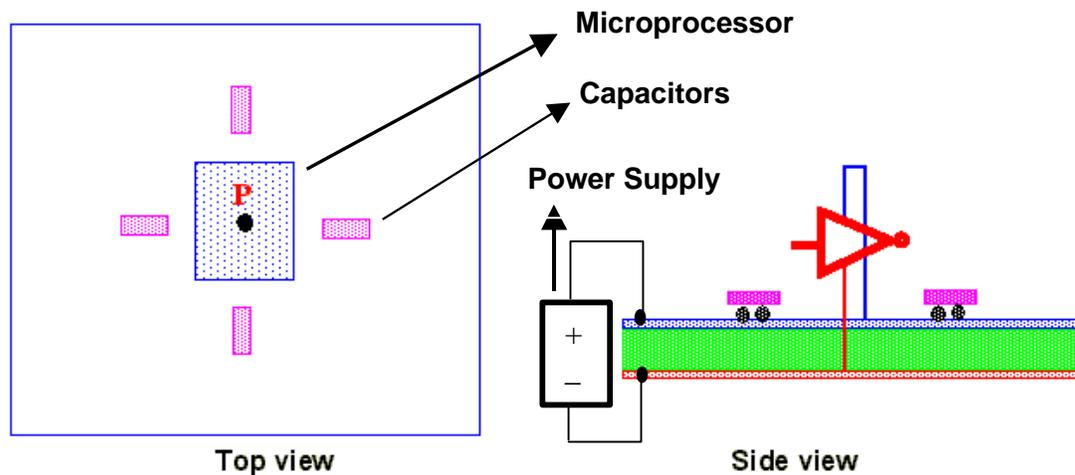
Figure 5.13 Layout of the package
