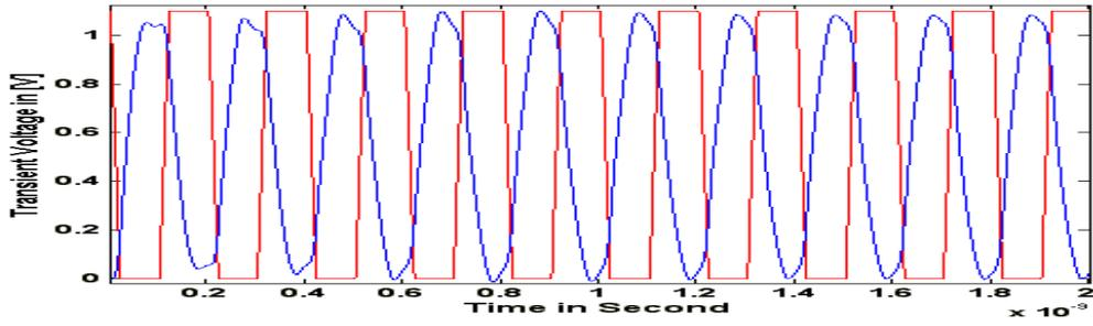
Figure 7.2(a) Input and output voltage of the driver
