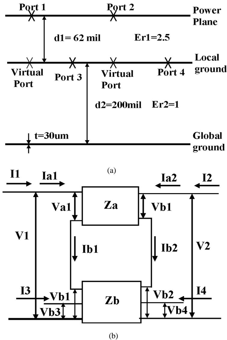
Figure 5.6 (a) Plane coupling through ports
