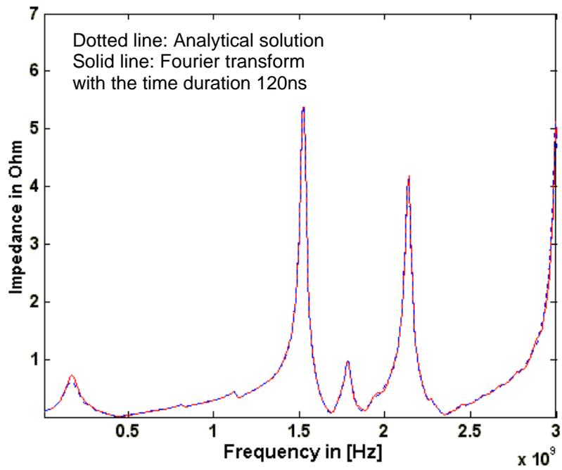
Figure 6.9(b) Comparison of the frequency response
