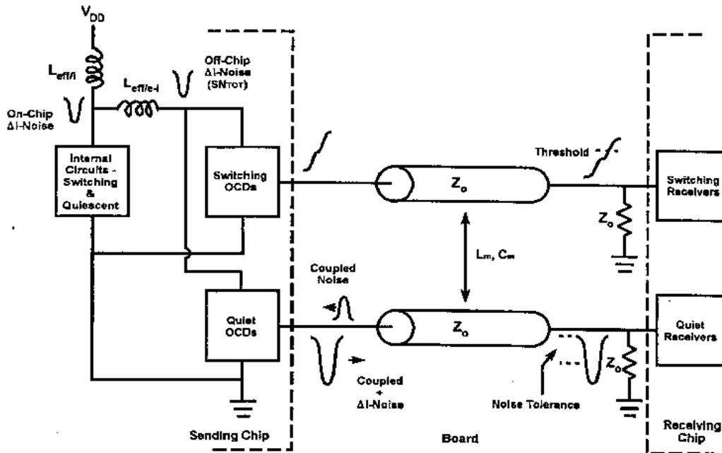
Figure 1.3. Causes and effects of Switching and Coupled Noise on Signal Lines[10]
