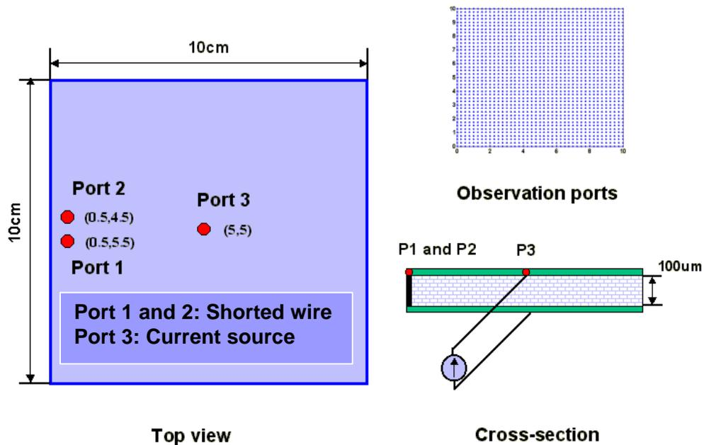
Figure 6.10 Plane pair for the radial wave propagation
