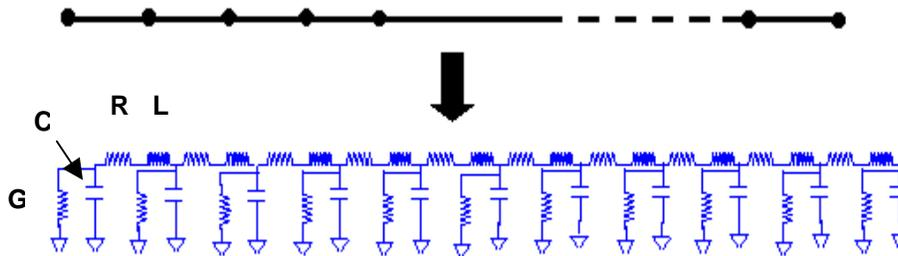
Figure 4.1 (b) Circuit representation of a transmission line with  $p$  model
