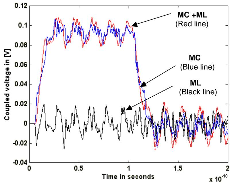
Figure 4.5(c) Far-end noise responses at node 3, with mutual capacitance only, mutual inductance only and mutual capacitance and inductance coupling
