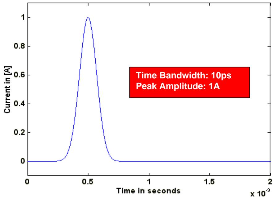
Figure 2.7(a) Gaussian current pulse used for the simulation
