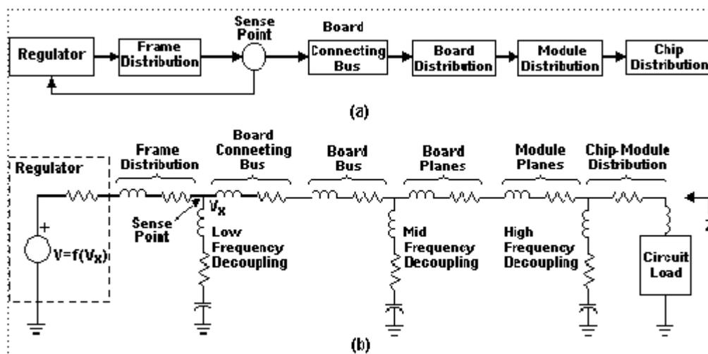
Figure 1.1.(a) Block diagram for typical power distribution system
