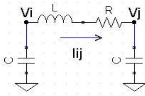
Figure 2.1  $p$ -type equivalent circuit of a small-sectioned transmission line
