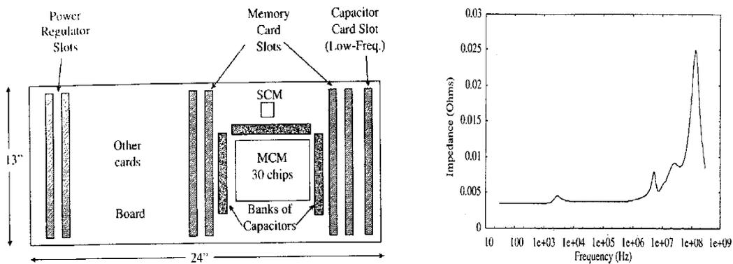
Figure 1.2. Layout of the back-plane of a system and the impedance seen from the chip circuit
