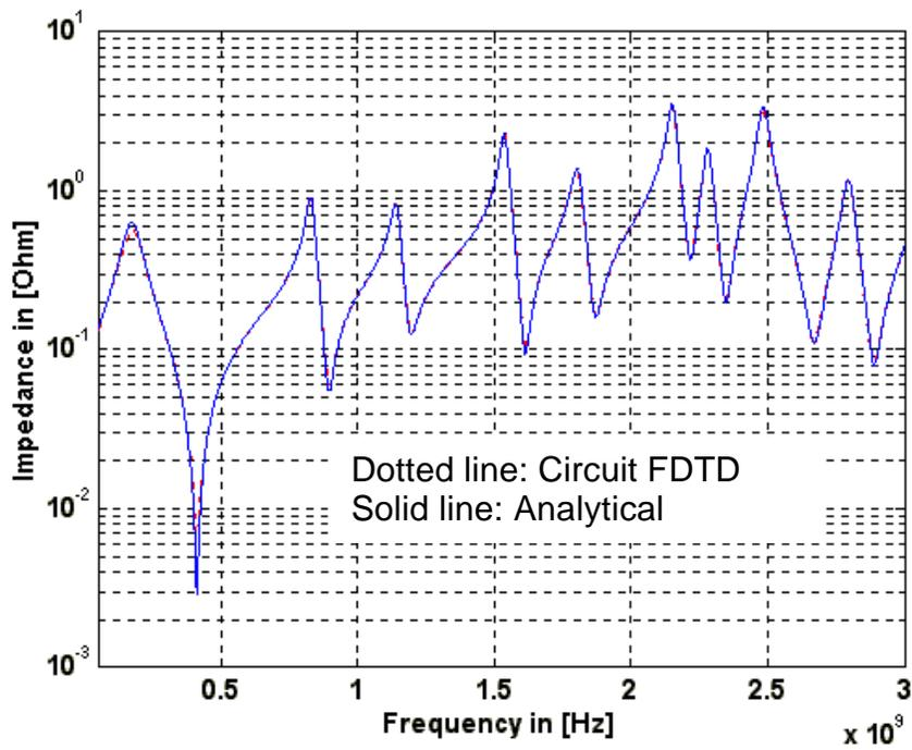
Figure 6.7(b) Self-impedance at Port 2 from the shorted structure
