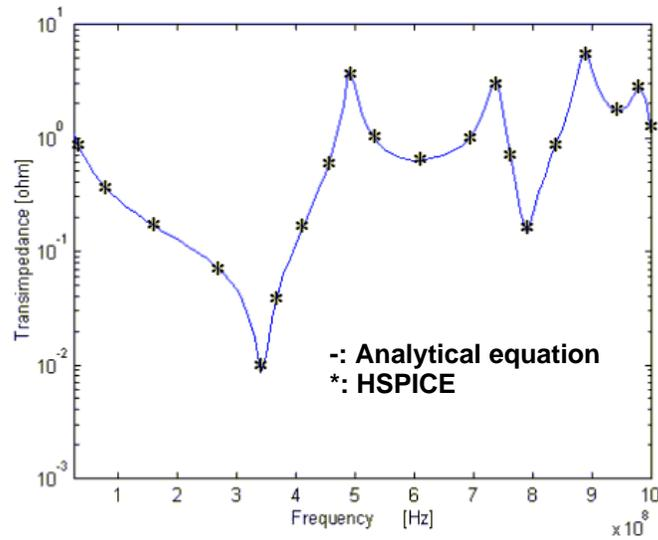
(a) Transfer-impedance with no decoupling capacitor
