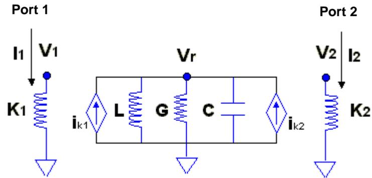
Figure 6.1 (b) Detailed circuit information of the resonator circuit
