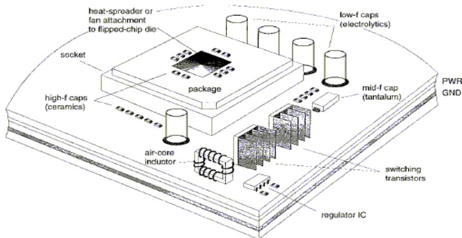
Figure 5.1 Power distribution network to a microprocessor
