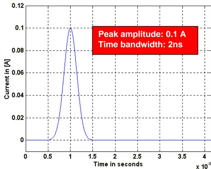
Figure 6.7(a) Gaussian pulse used for the frequency response
