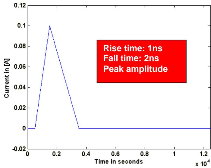
Figure 6.6(a) Wave form of the current source at Port 2
