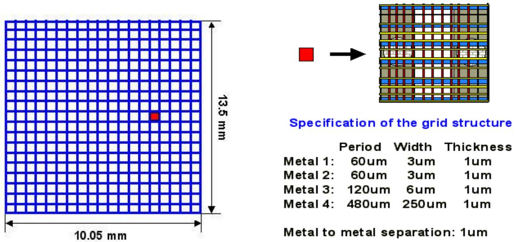
Figure 2.4(a) On-chip power grid structure (b) Detailed description of a unit cell
