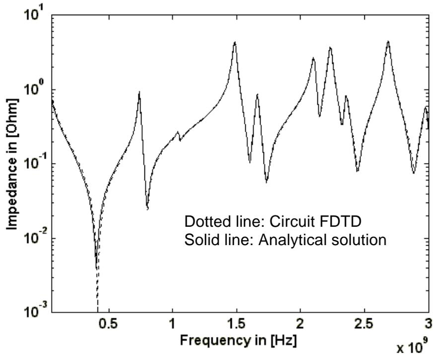
Figure 6.8 (a) Self-impedance at Port 2 from the open structure
