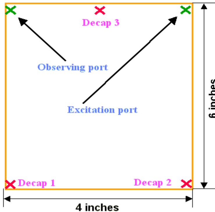
Figure 5.11 Plane structure with 3 decoupling capacitors
