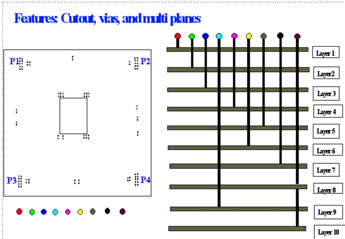
Figure 5.8 Top and side view of the ceramic test vehicle
