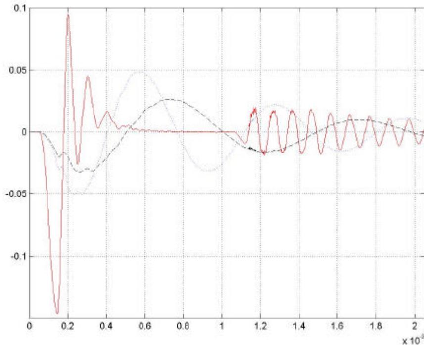
Figure 3.6 Differential noise waveforms with the different decoupling capacitors
