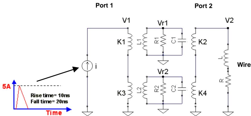
Figure 6.3 A test resonator circuit
