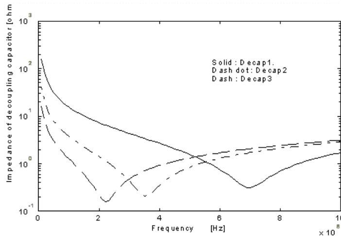
Figure 5.10 Frequency response of the decoupling capacitors
