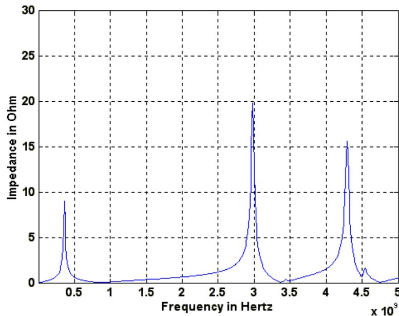
Figure 7.9 Self impedance seen from the port,2
