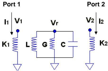
Figure 6. 1(a) A resonator circuit with two transformers
