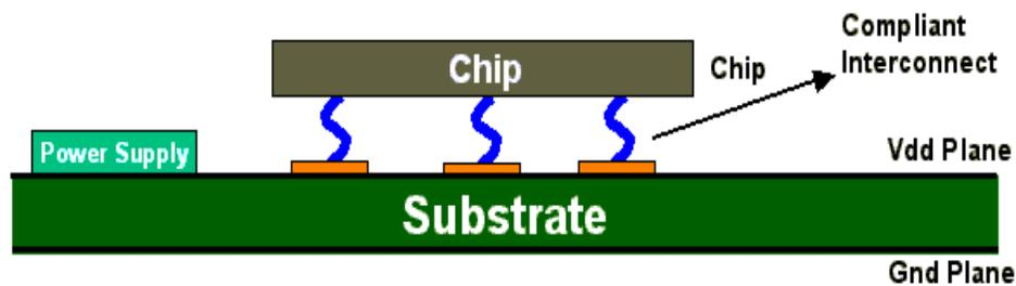
Figure 7.1 Wafer level package
