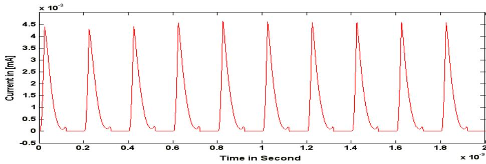
Figure 7.2(b) Current signature at a CMOS Inverter
