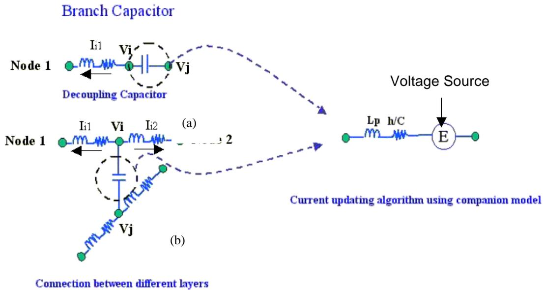
Figure 2.2 (a) Decoupling capacitor implemented as a branch capacitor
