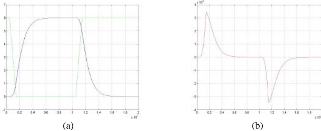
Figure 3.2 (a) Transient output voltage from FDTD and SPICE
