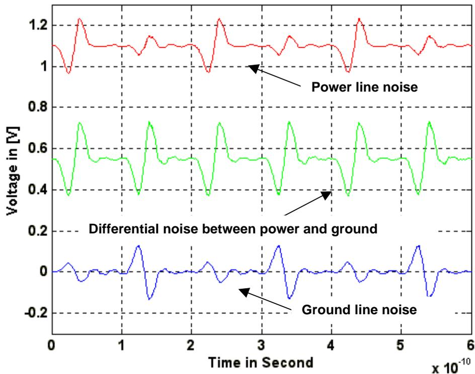
Figure 4.9 Power supply noise near the driver from Test Case 3
