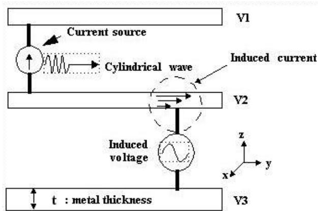
Figure 5.5 Skin effect approximation for plane-plane coupling
