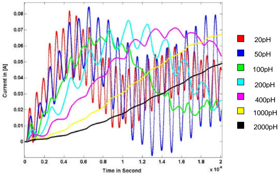
Figure 7.4 Current transient from the power grid structure with the variation of compliant interconnect inductance from 20pH to 2nH
