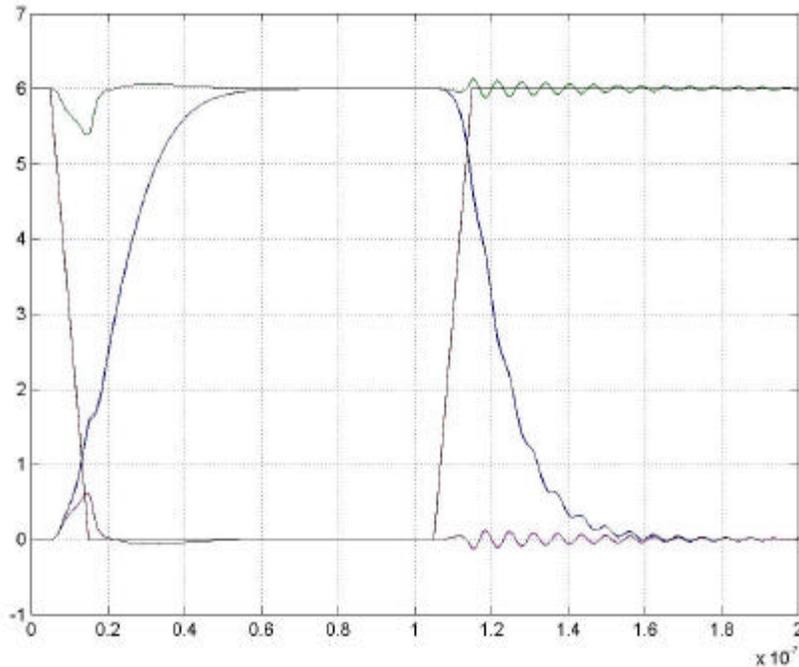
Figure 3.3(b) Transient voltage response and power and ground bounce
