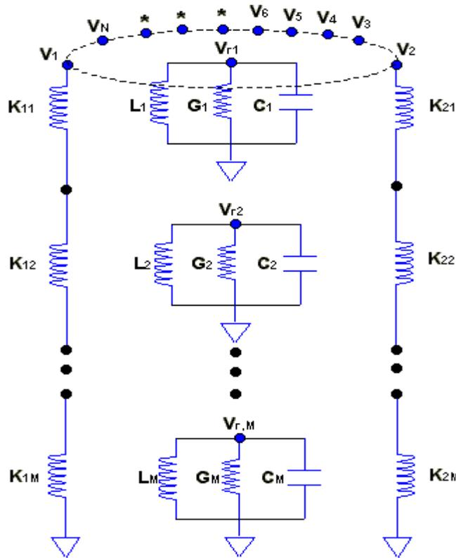
Figure 6.2. N-port coupled system with M resonators
