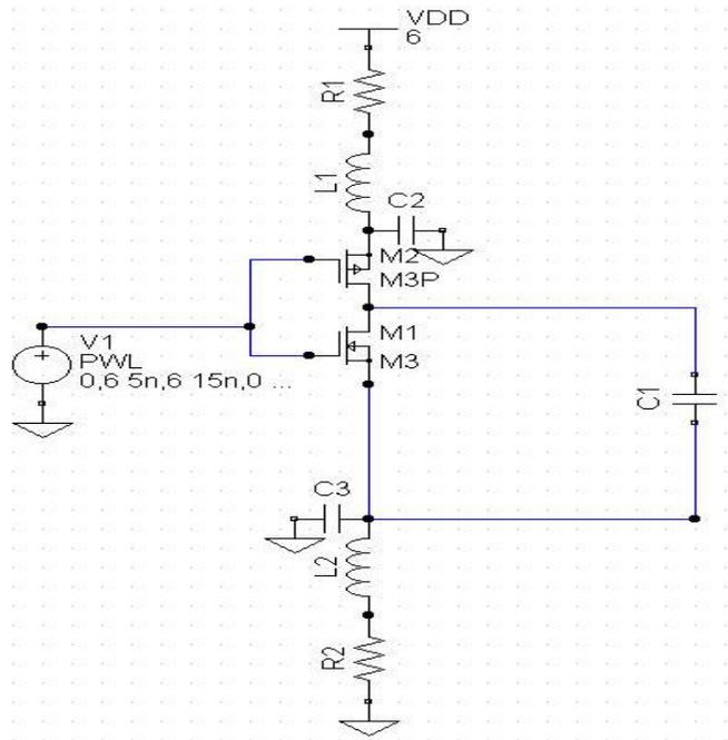
Figure 3.3 (a) CMOS inverter with some parasitic
