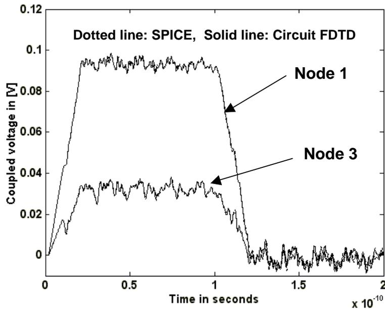
Figure 4.5(a) Near-end noise at nodes 1 and 3
