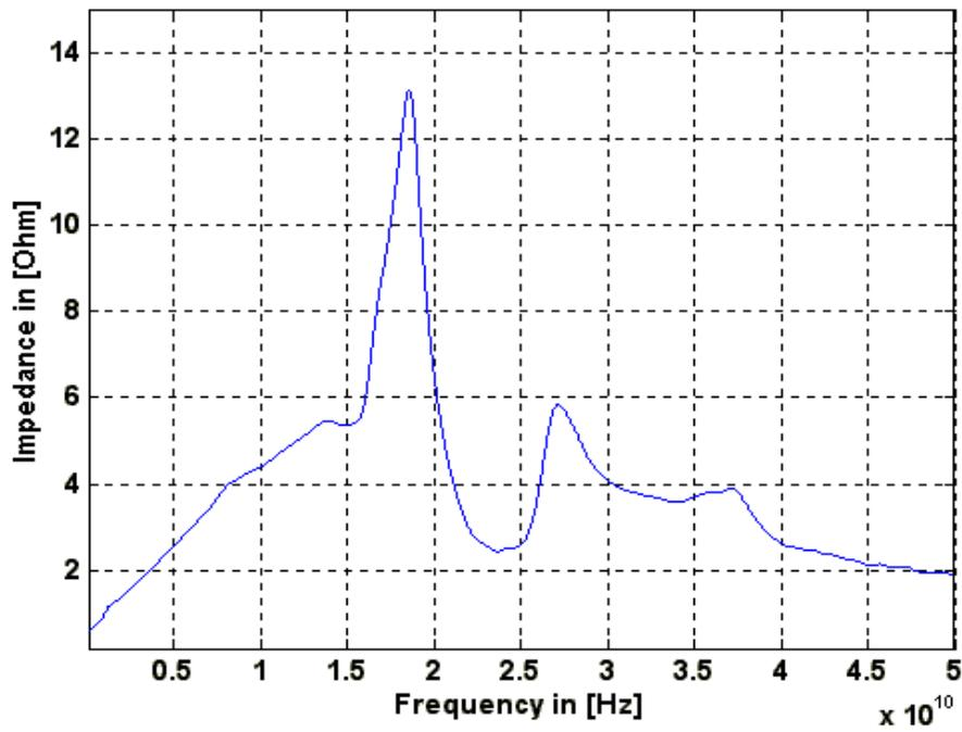
Figure 2.7(b) Self-impedance seen from the center of the on-chip power grid
