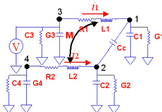
Figure 4.2 A simple coupled structure
