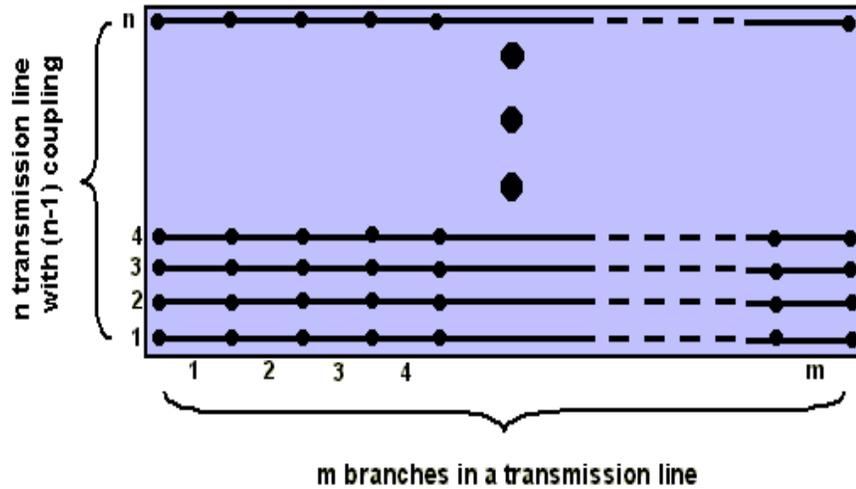
Figure 4.1(a) n transmission lines with (n-1) couplings over a ground plane
