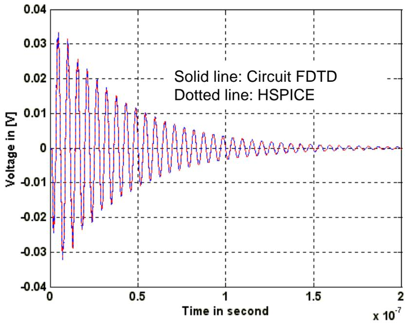
Figure 6.6(c) Coupled noise at Port 3 due to the current source at Port 2
