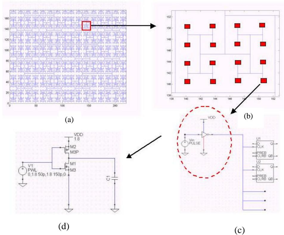
Figure 3.4(a) H-tree based clock network (b) Enlarged part of the clock network
