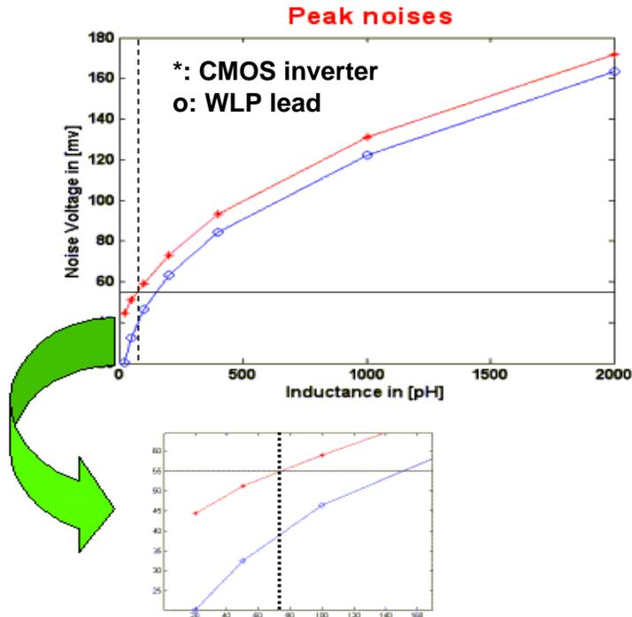
Figure 7.5 Peak noise at the location of CMOS inverters and compliant interconnect
