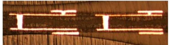
Fig. 1 Cross section of ultra thin RXP substrate
