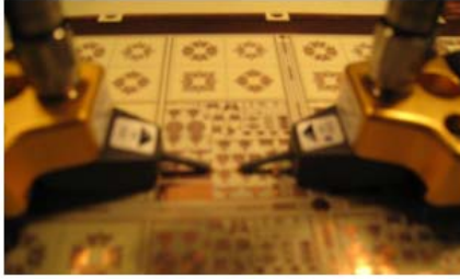
Fig. 10 Measurement equipment with GSG probes
