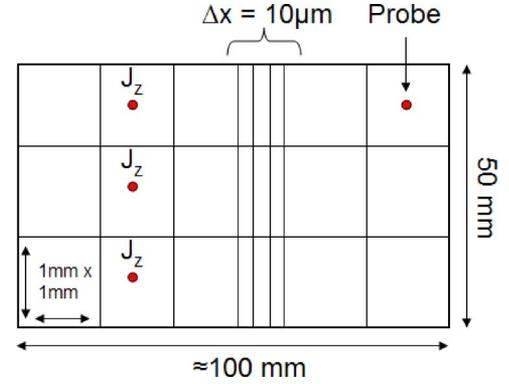
Fig. 6. Test case 1. Solid power plane structure with a nonuniform mesh.
