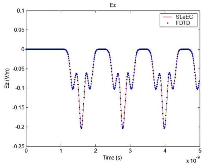
Fig. 7. Simulation results from 0 to 5 ns for test case 1. (Red, solid line) SLeEC. (Blue, dotted) FDTD.
