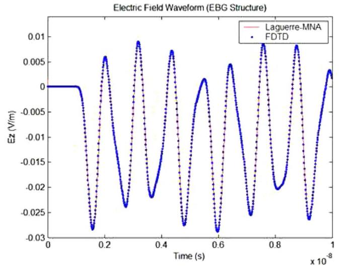
Fig. 10. Simulation results from 0 to 10 ns for test case 2. (Red, solid line) SLeEC. (Blue, dotted) FDTD.
