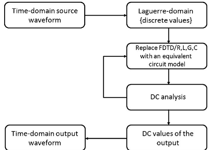
Fig. 2. Flowchart for transient simulation using Laguerre polynomials.
