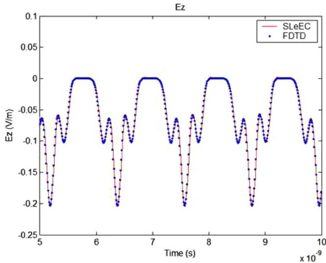
Fig. 8. Simulation results from 5 to 10 ns for test case 1. (Red, solid line) SLeEC. (Blue, dotted) FDTD.
