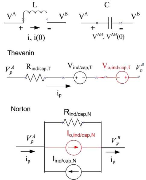
Fig. 5. Thevenin/Norton form of the companion model for an inductor/capacitor.
